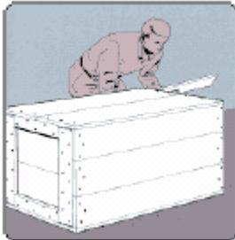
4. Reinforce the boxes with adequate tension metal straps placed one-sixth of the distance from the ends, unless containers are in excess of 48 inches in length or over 250 pounds. Then three or more straps should be used, with one for each additional 24 inches. Staples should be used to hold strapping in place when boards are five-eighths of an inch in thickness or greater.
